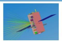
The accurate estimation of the dose received in orbit by electronic components requires the consideration of the system 3D geometry.
