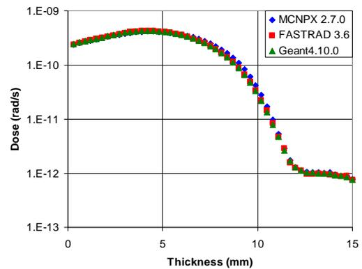
Fig. 2, Deposited dose in Aluminum layers according to the crossed thickness for: MCNPX (blue diamond), FASTRAD (red square), and GEANT4 (green triangle).
