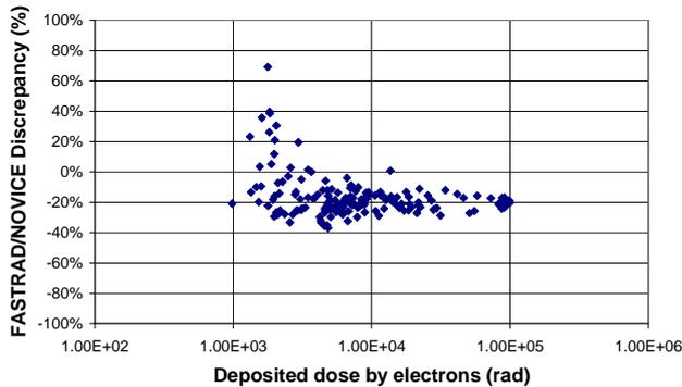
Fig. 9, FASTRAD/NOVICE discrepancy according to the deposited dose in FASTRAD for trapped (blue line) electrons, only considering the transmitted electrons.
