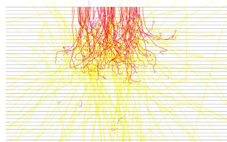
Fig. 1, 5 MeV electron beam incident on successive aluminum layers. Primary electrons are shown in red, secondary electrons are shown in magenta, and secondary photons are shown in yellow.
