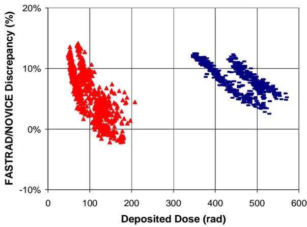
Fig. 7. FASTRAD/NOVICE discrepancy according to the deposited dose in FASTRAD for trapped (blue line) and solar (red triangle) protons. 641 point detectors have been used for the comparison.
