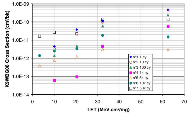
Fig. 6. Samsung memory SEU cross section
