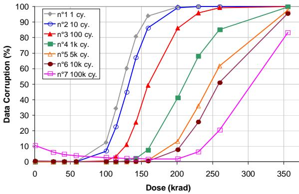
Fig. 1. Data corruption versus TID level – Samsung memory
