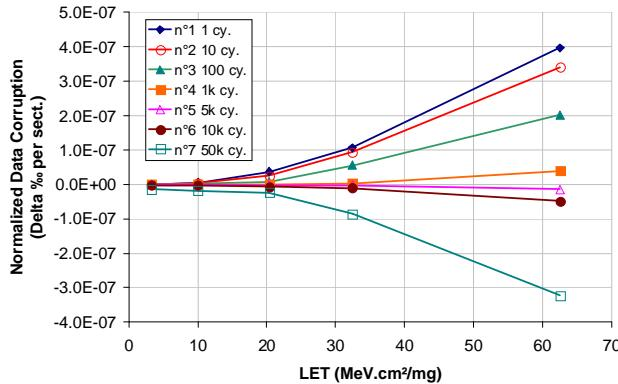
Fig. 3. Normalized Data Corruption versus LET – Samsung memory
