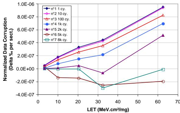
Fig. 4. Normalized Data Corruption versus LET – Micron memory
