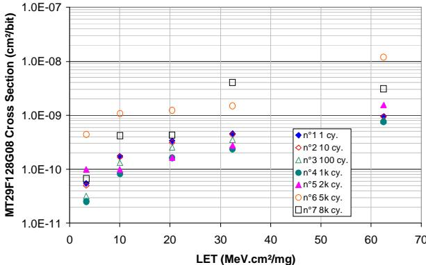
Fig. 7. Micron memory SEU cross section
