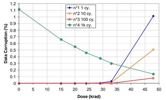
Fig. 2. Data Corruption versus total dose – Micron memory
