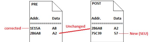
Fig. 5. SEE post-analysis principle
